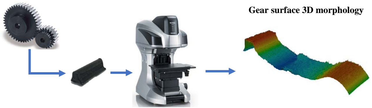
Figure 9 Demonstration of the process of obtaining the surface morphology feature during the gear wear propagation
