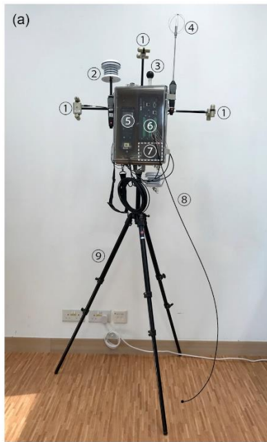
Fig. 5. An example of the self-developed weather monitoring systems: (a) the stationary station type; (b) the type for mobile measurement.
