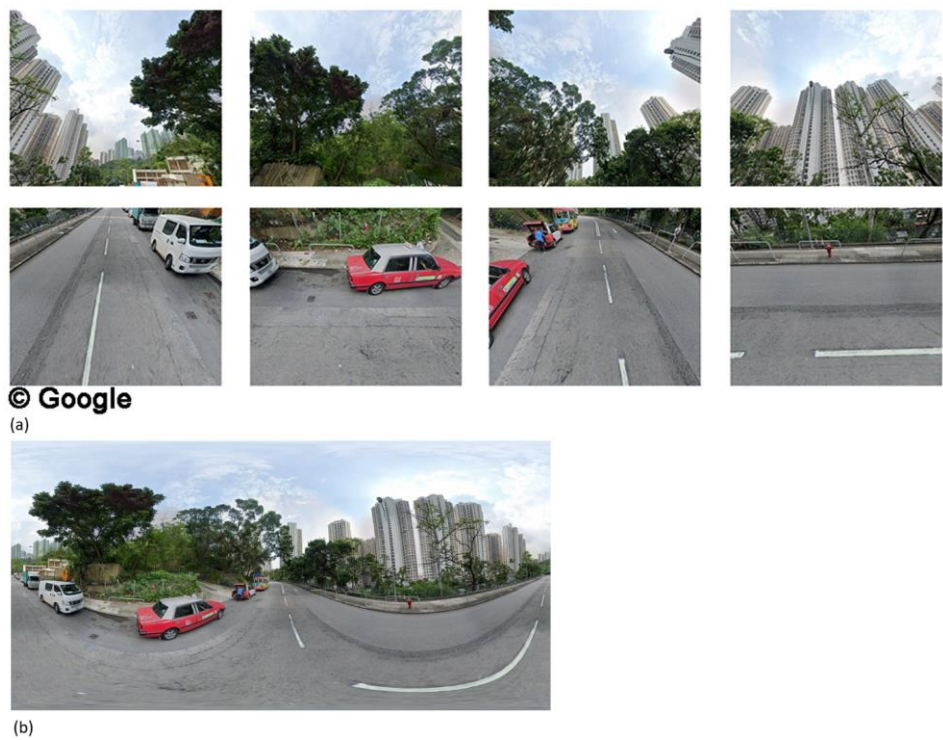
Fig. 2. GSV image collection and processing at a point: (a) eight images captured from four directions and two angles and (b) panorama
