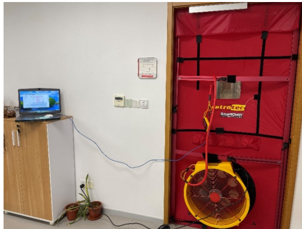
Figure 2: The blower door test system
