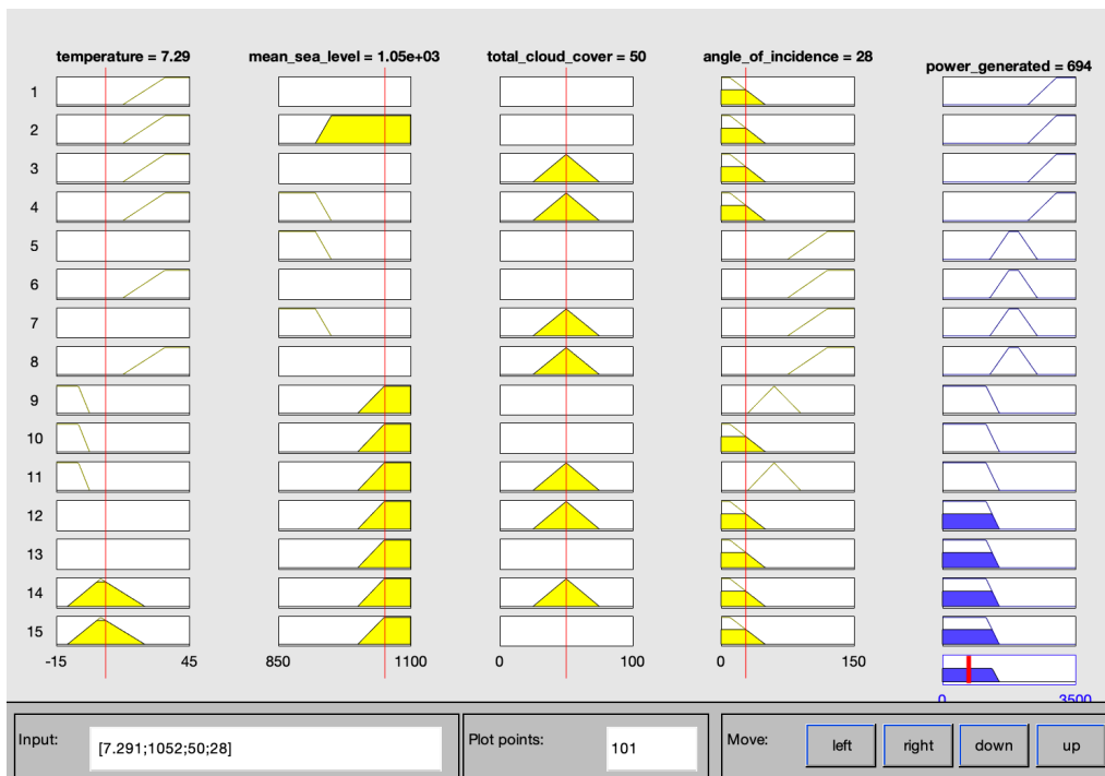
Fig. 4. An example of generating solar energy prediction based on the integrated model
