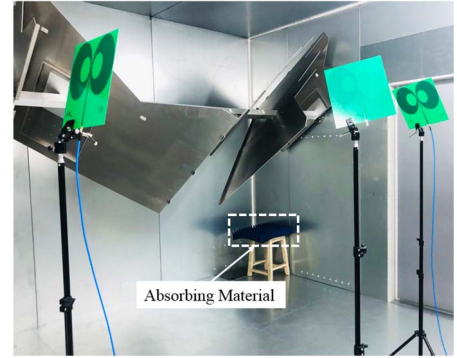
Fig. 8. Antenna efficiency measurement (with absorbing material) in reverberation chamber.
