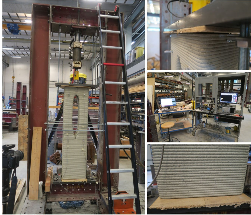
Figure 33: The setting of the structural load test
