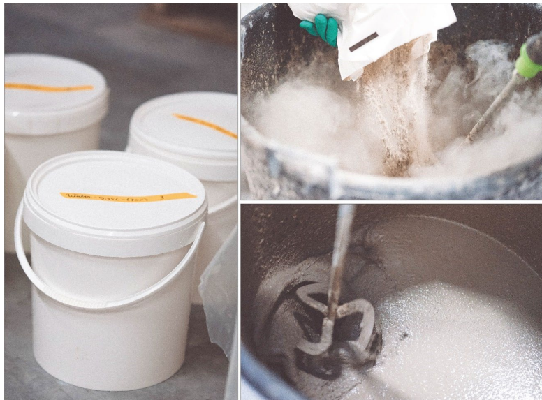
Figure 26: Preparing and mixing the self-compacting concrete
