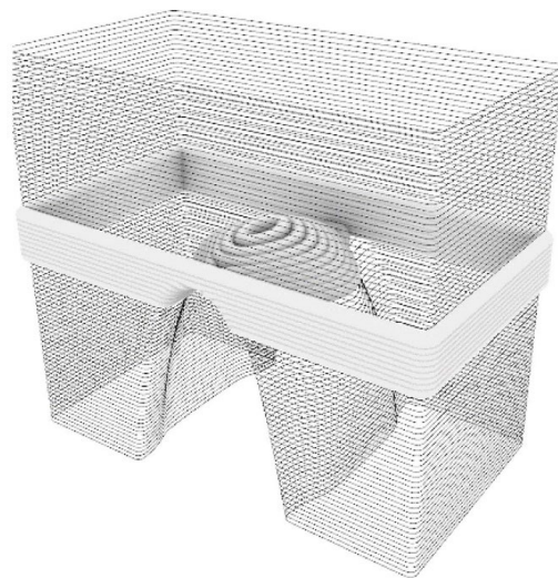
Figure 9. Illustration of a watertight model with overhangs at the centre of the column as a result of topology optimisation
