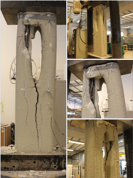
Figure 39: Demonstrating the failure mode of the 1:3-scale prototype after load testing
