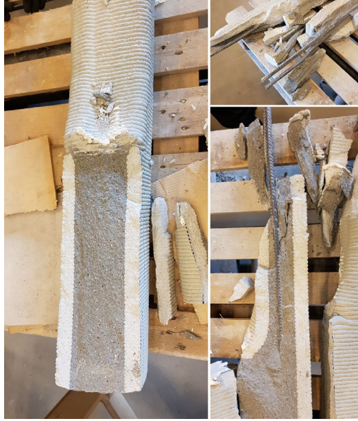
Figure 40: After removal from the compression machine. Light grey shows the printed concrete, and dark grey shows cast concrete
