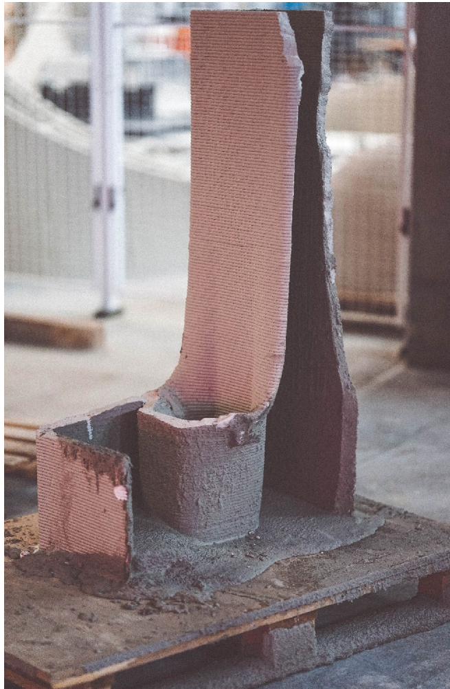
Figure 32: Controlled demolition showing adhesion of the 3D concrete printed layers
