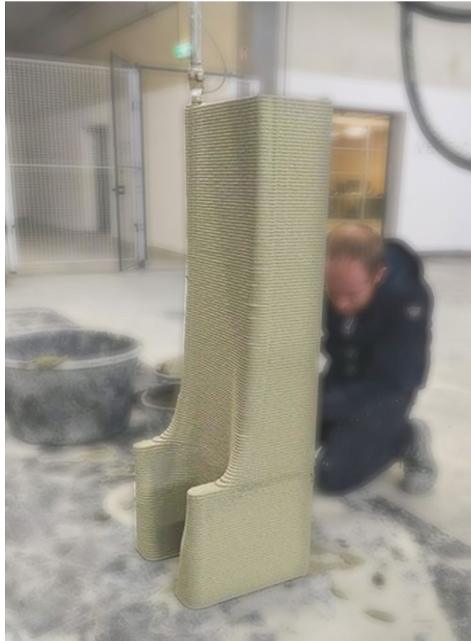
Figure 19: Printing a full-scale fragment
