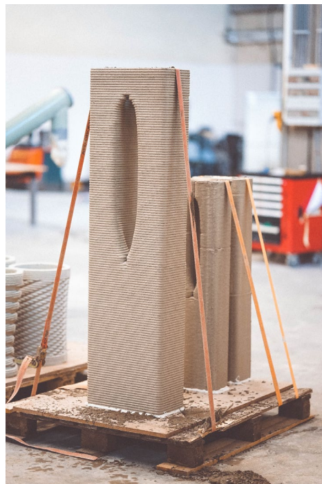
Figure 18: Prototypes of the scaled columns (1:2-scale in the foreground and 1:3-scale in the background)
