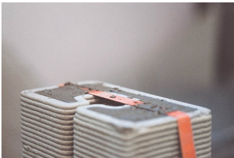
Figure 28: Completed reinforced concrete prototypes
