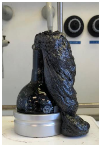
Figure 1.6 An example of auto-acceleration in the inverse vulcanisation.
