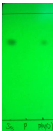
Figure 4.28 TLC results of detecting free elemental sulfur in poly(S-CDE) Spots on baseline are sulfur, poly(S-CDE), and the product made absence catalyst.
