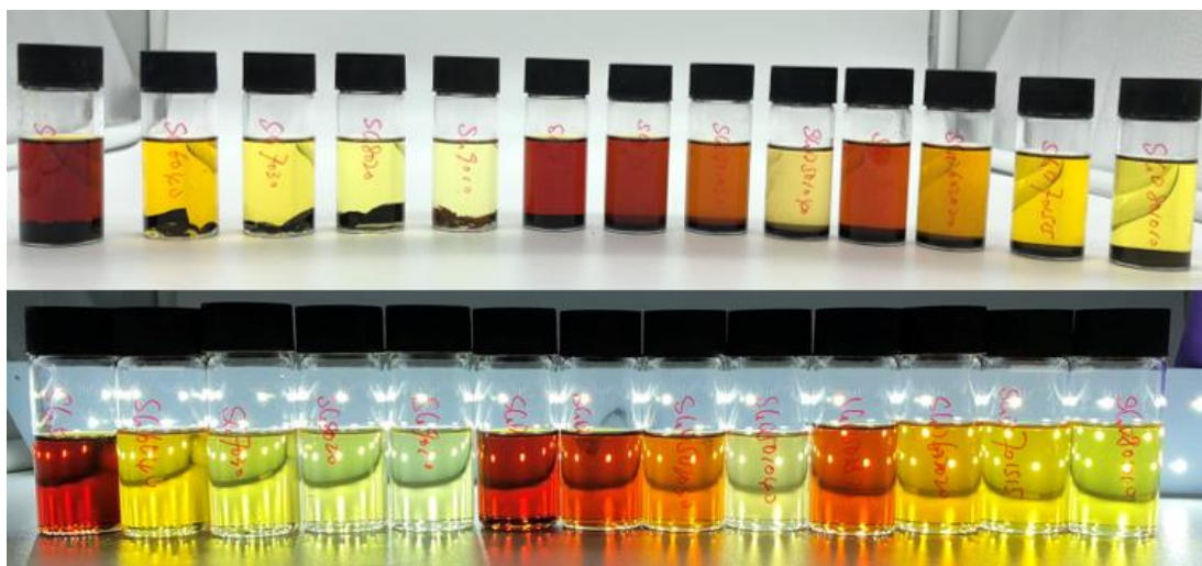
Figure 3.10 Solubility study of polysulfides. (top) and soluble fractions in \text{CHCl}_3 (bottom). From left to right, they are SG5050, SG6040, SG7030, SG8020, SG9010, SGD504010, SGD503020, SGD502030, SGD501040, SGD502525, SGD602020, SGD701515, and SGD801010.
