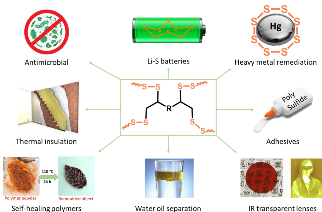
Figure 1.7 Different potential applications of inverse vulcanised polymers.
