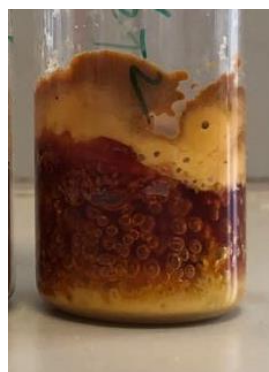
Figure 4.2 It can be observed that sample SDIB30C1T110 is inhomogeneous with bubbles, which is because of low mobility of the system followed by triggering auto acceleration.
