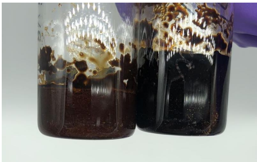
Figure 4.24 Photo of poly(S-CDE) made with and without catalyst. Left sample is the product without catalyst (lighter in colour) and right one is poly(S-CDE) made adding 10% NaDTC (darker)
