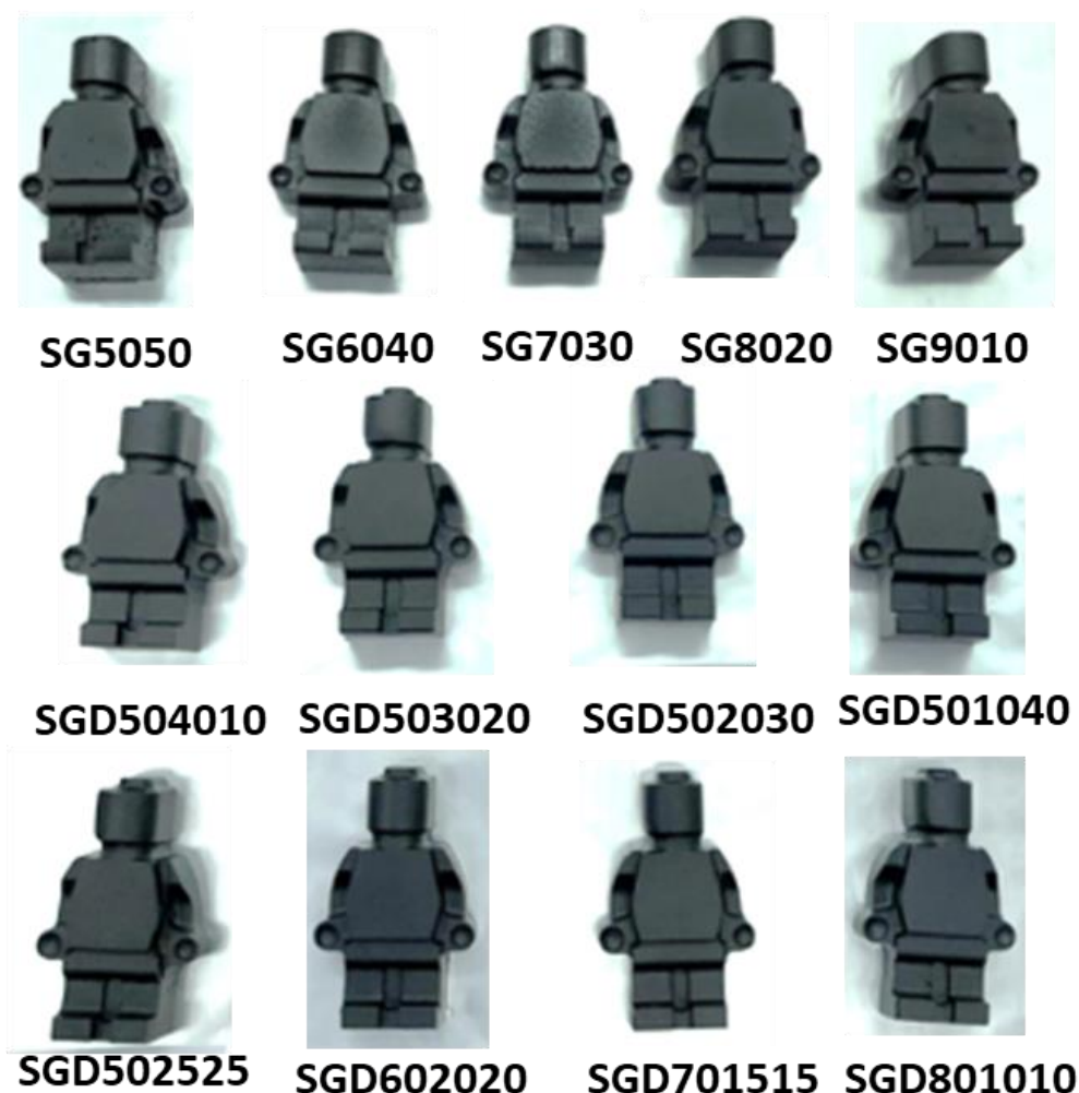
Figure 3.1 Photographs of final molded products of different polysulfides after curing. The dimension of the samples is 25 mm × 40 mm.
