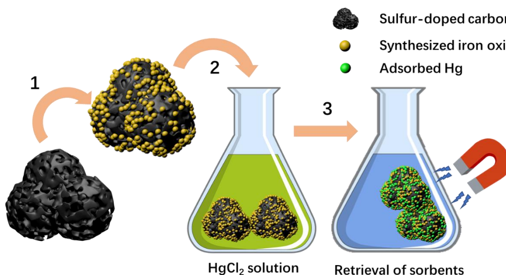
Figure 5.1 Schematic of synthesis procedure of magnetic sulfur-doped carbons and the application of magnetic sulfur-doped carbons for mercury adsorption. Step 1. Functionalization of sulfur-doped carbons from precipitation of iron oxides onto sulfur-doped carbons surface. Step 2. Removal mercury from mercury chloride solution. Step 3. Retrieval of sorbents after adsorption via a magnet.
