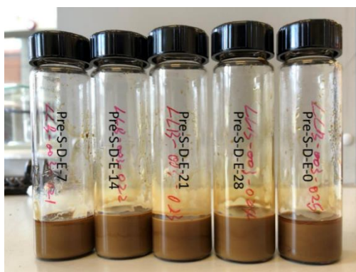
Figure 2.5 Reserved prepolymers ready for delayed curing
