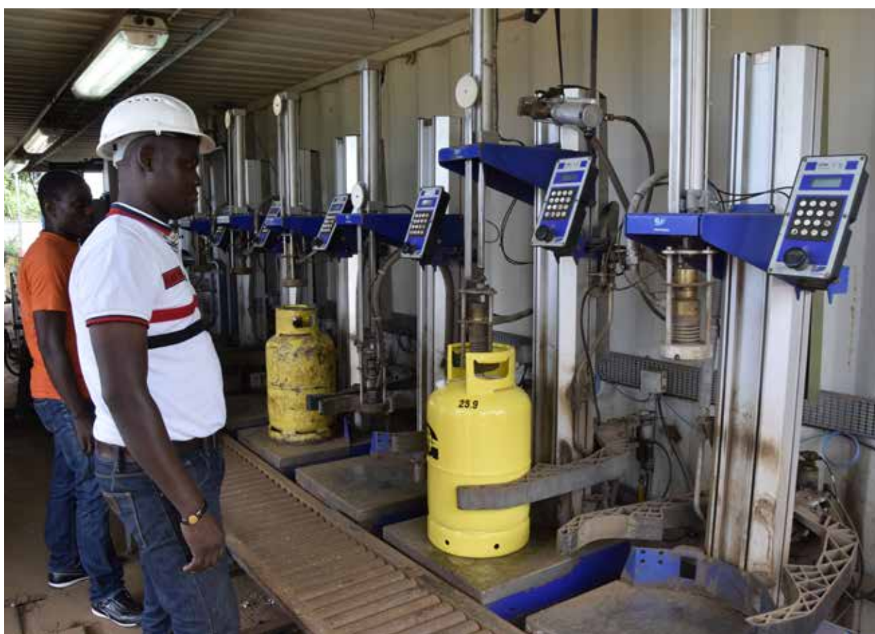
LPG cylinder filling. Photo credit: Nigel Bruce
