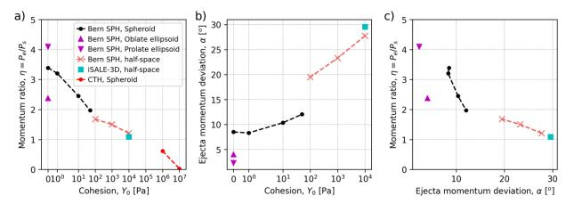
Figure 4: Results from numerical simulations of impacts, at  $i = 45^{\circ}$ , from Bern SPH, iSALE-3D and CTH. a) Ratio of the ejecta momentum to the impactor momentum ( $\eta$ ) as a function of target cohesive strength. b) Ejecta momentum direction from the normal,  $\alpha$ , as a function of cohesion. c) Momentum ratio  $\eta$  as a function of ejection angle  $\alpha$ .
