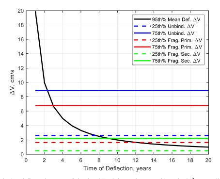
Figure 7:  $\Delta v$  required to deflect a large set of simulated Earth-impacting asteroids at the 95<sup>th</sup> percentile level as a function of time of deflection prior to Earth encounter. The horizontal lines show the  $\Delta v$ , at the 25<sup>th</sup> and 75<sup>th</sup>
