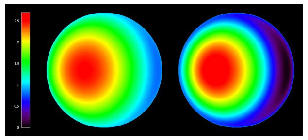
Figure 5: Spacecraft's view of an idealized spherical asteroid showing a map of  $\beta_u$  across the surface. Values are indicated by the color scale at far left. The desired deflection direction  $\hat{u}$  is into the page and 40° to the right. (a), left: ejecta response Model 1, equation (23); (b), right: ejecta response Model 2, equation (24).
