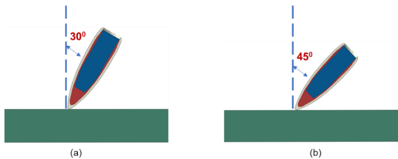
Figure 20. FE model set up for oblique impact (a) 30° impact (b) 45° impact
