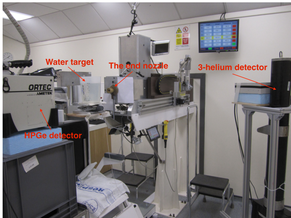
Figure 7.1: Photograph of the treatment room. The HPGe detector and the 3-helium detector were aligned with the beam axis using supported materials and placed at different angles from the beam axis.
