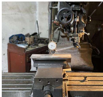
Fig. 3. Setup for initial local geometric imperfection measurements.
