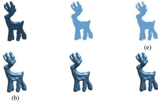
Fig. 2. Illustrations of (a) input 109 slices with 1 gap; (b) output from (a); (c) input 55 slices with 3 gaps; (d) output from (c); (e) input 37 slices with 5 gaps; (f) output from (e).
