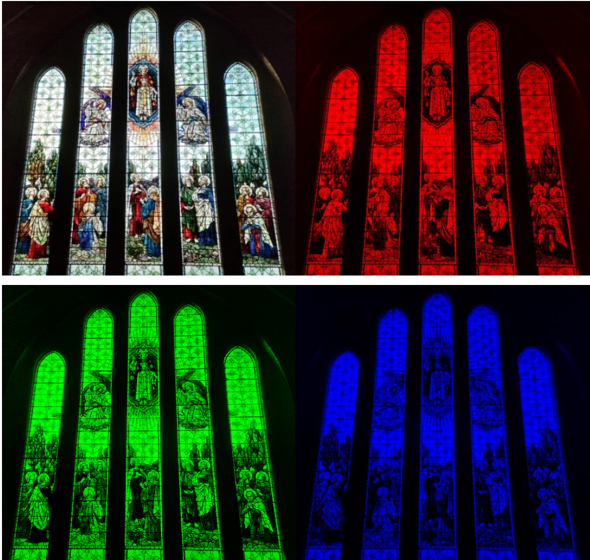
Figure 2.5: Example image showing the original image (top left) and the image broken down into red, green, and blue channels.
