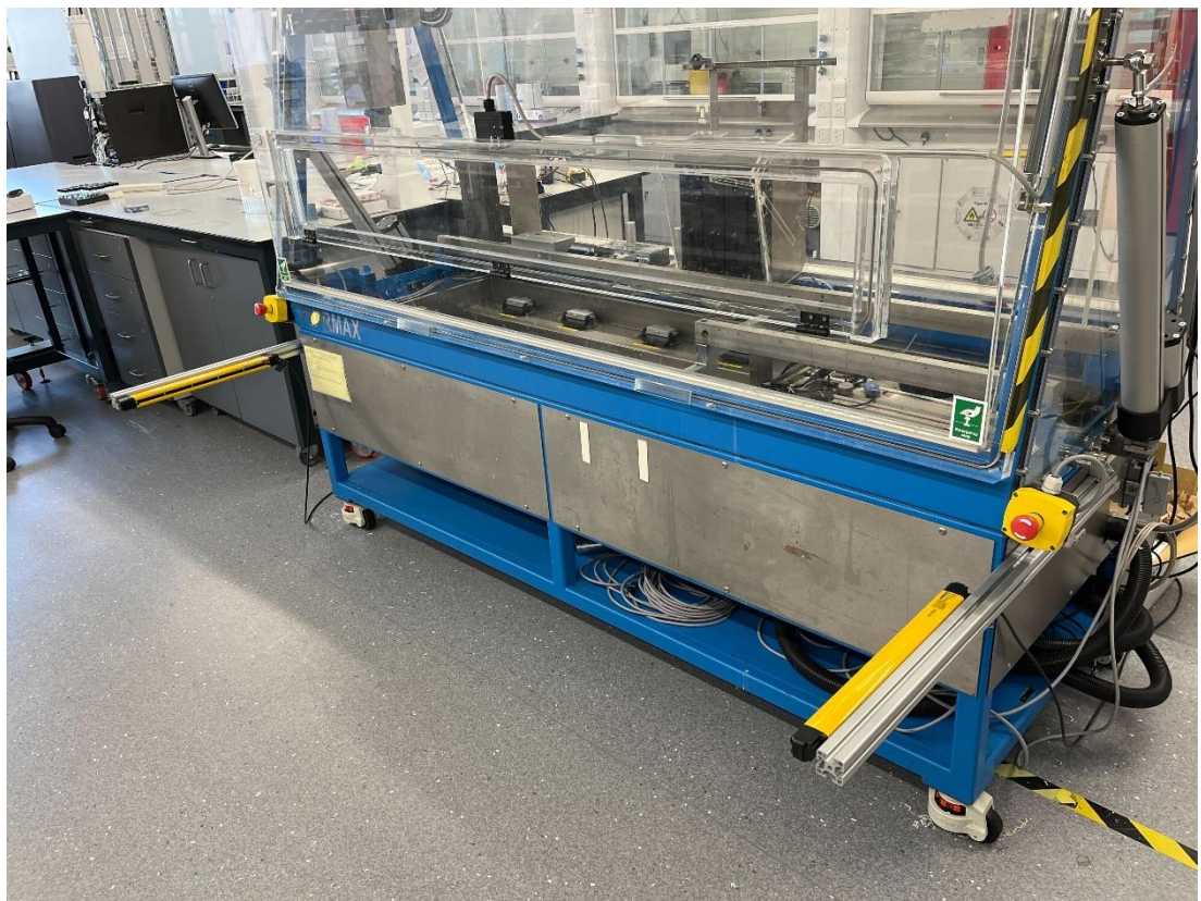
Figure 4-5: Extruded aluminium framework for supporting light curtains.
