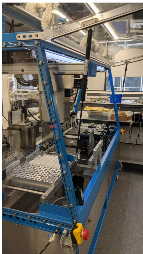
Figure 4-2: Unmodified ChemSpeed ISynth platform (above), Hinge mechanism and hydraulic supports (lower).
