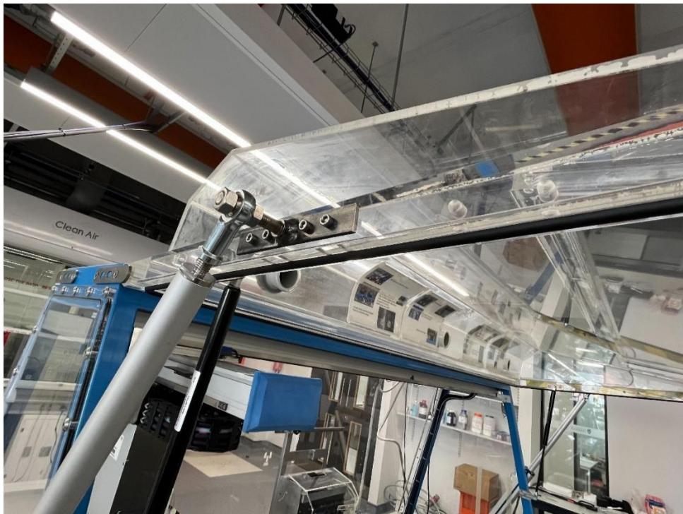
Figure 4-3: Metal fittings for mounting linear actuators to side of Formax housing (upper); Brackets for attaching end of actuators to side of Formax hood (lower)
