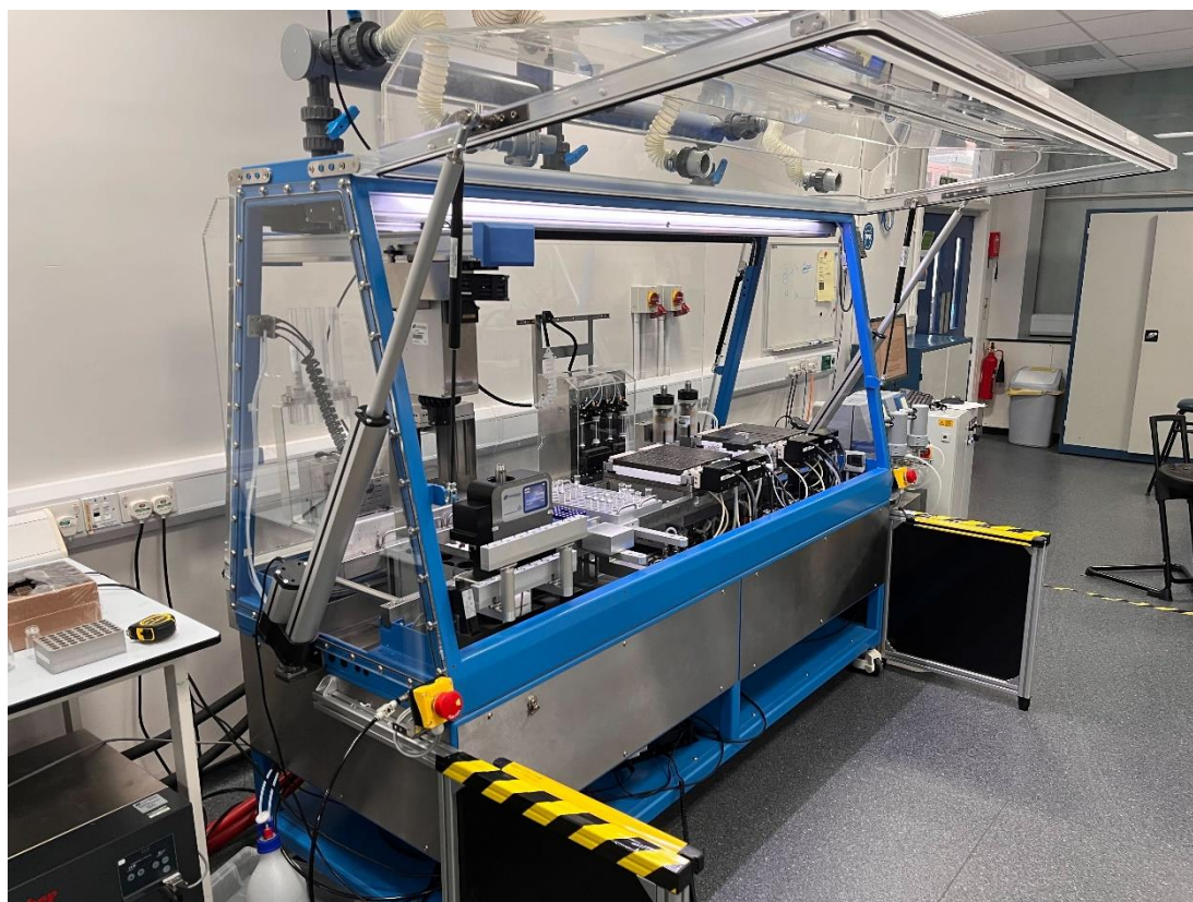
Figure 4-6: Fully constructed actuator and light curtain system installed on ISynth platform.
