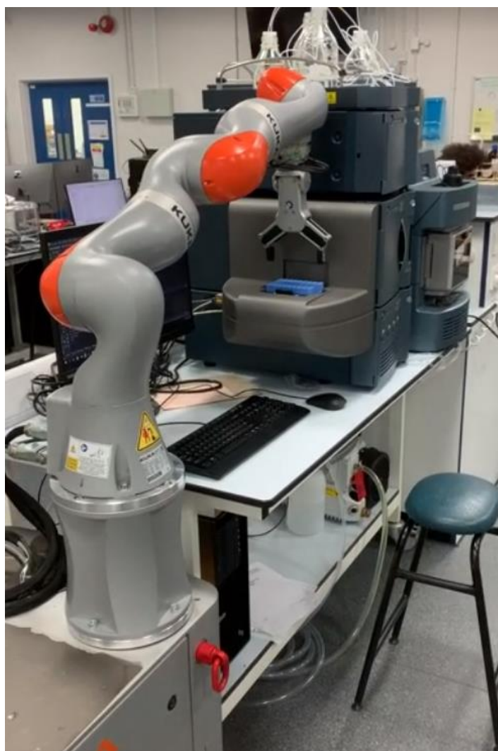
Figure 4-8: Automation Portal (side view) for insertion of LC-MS racks.
