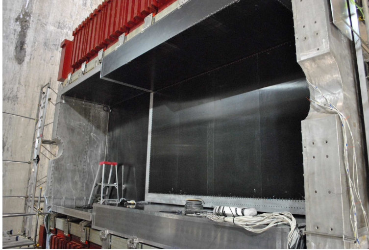
Figure 3.1: One side of the ECal installed within the ND280 magnet. Three of the six barrel-ECal modules can be seen on the right, with three of the thinner PØD-ECal modules on the left. The basket, which contains the DS-ECal, is not present [72].
