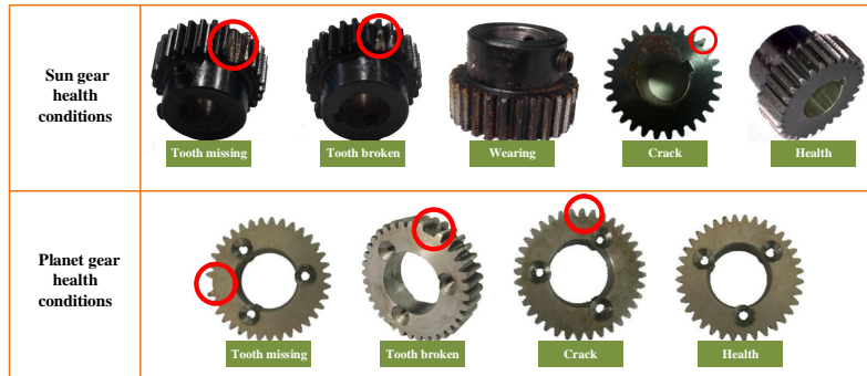
Figure 7: The different health conditions of the sun gear and planet gear.
