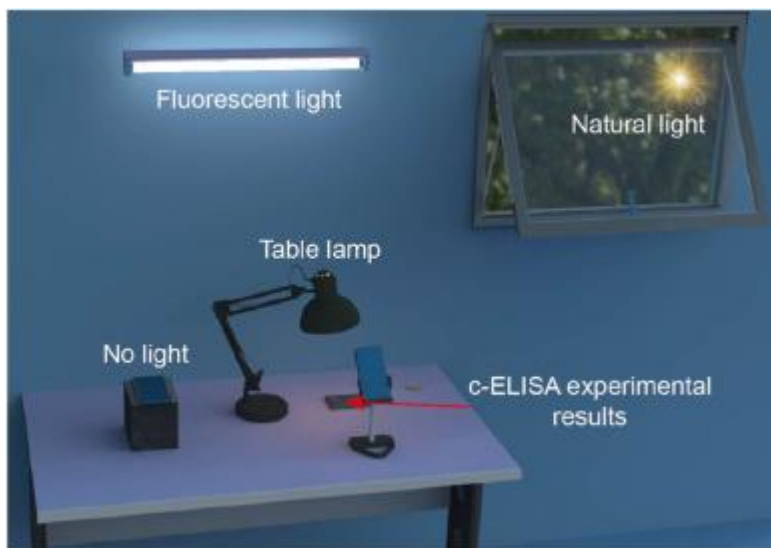
Fig. 3. Schematic illustration of an image captured with a smartphone camera under no-light conditions and different combinations of fluorescent light (F), table lamp (L), and natural light (N) conditions.
