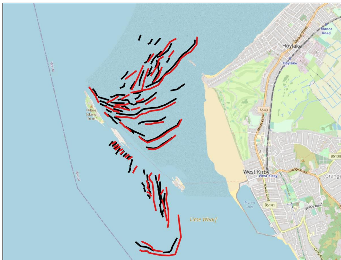
Figure 5.9: Lines indicating maximum deposition from LiDAR differences; 2007 and 2006 (black), 2008 and 2007 (red), showing progression of sand features in a shoreward direction.
