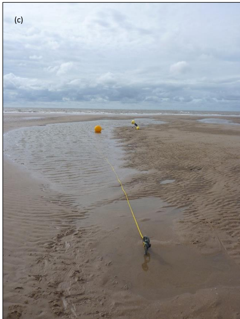
Figure 4.1: (a) Top part of mooring together with the GNSS buoy, (b) ground anchor with swivel, (c) complete mooring installed and laid out on the beach at low water.
