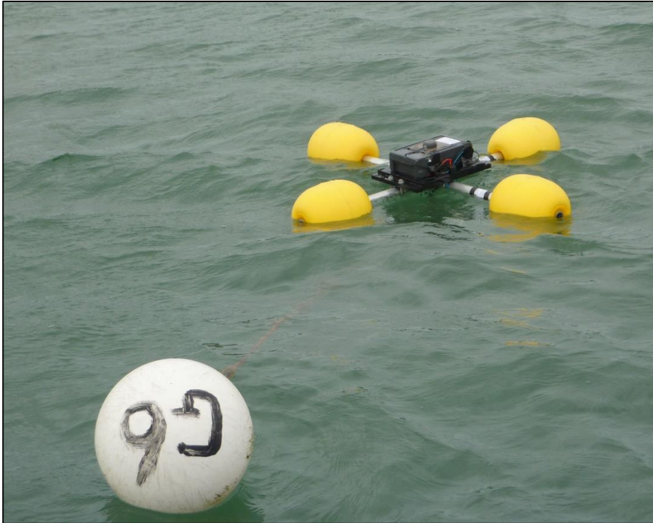
Figure 2.3: GNSS buoy attached to mooring buoy in Holyhead New Harbour.
