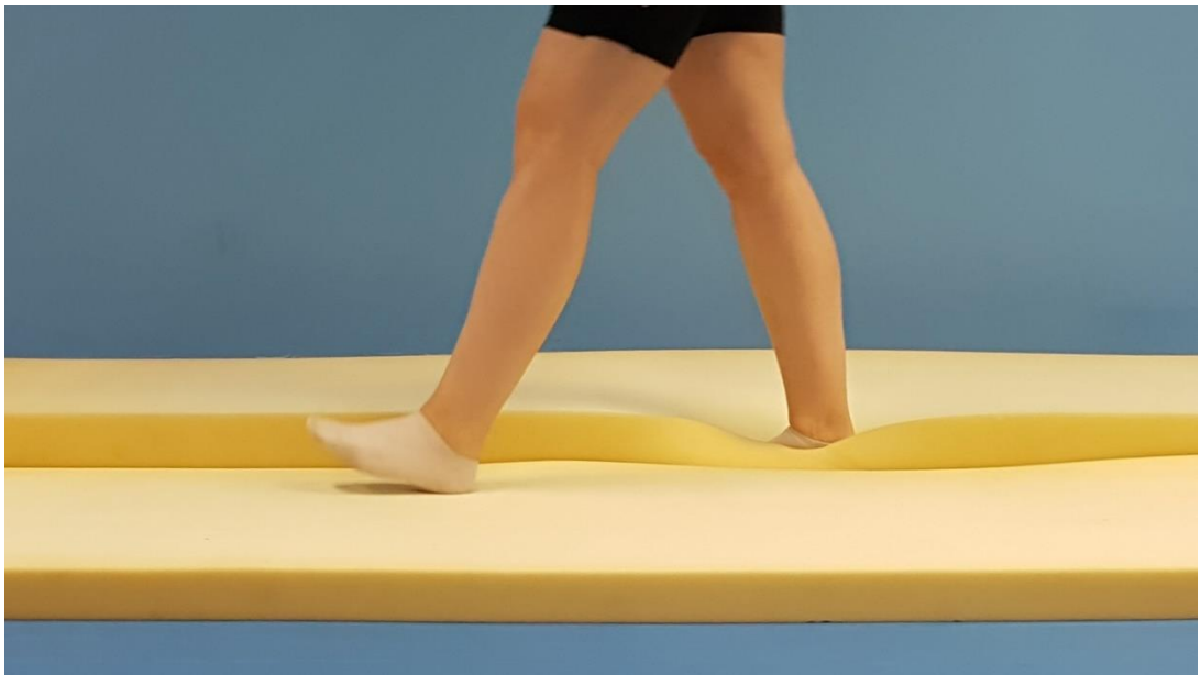
Figure 2.1: Example of the compliant substrates: 13cm “thick” compliant foam (back) and 6cm “thin” compliant foam (front).
