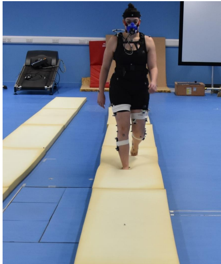
Figure 2.3: Example of walking on thin foam substrate placed over 3 in-series force plates with kinematic markers, sEMG sensors and a K5 wearable metabolic unit measuring oxygen uptake ( \dot{V}_{O_2} , ml s -1 ) and carbon dioxide produced ( \dot{V}_{CO_2} , ml s -1 ).
