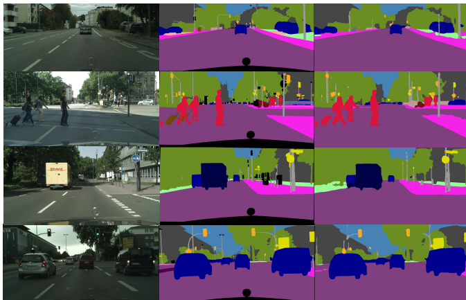
Fig. 6: Results of the proposed LGCNet on the Cityscapes validation set. The first column is input image, the second column is ground truth, and the final column displays the output of LGCNet.
