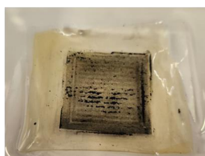
Figure S5. Photographs of A) Pre-run TiO 2 -loaded Nafion 117 and Sustainion X37-50 membranes and B) the assembled Nafion/TiO 2 /Sustainion membrane after 3 h operation at 100 mA cm -2 .
