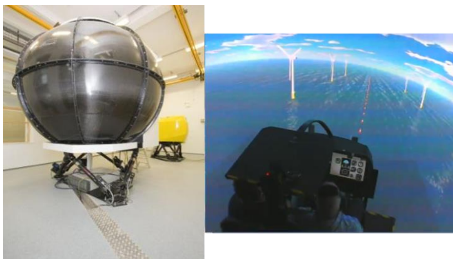
Figure 4-1: Left: HELIFLIGHT-R Flight simulator. Right: Cockpit interior and wind turbine farm scenario.
