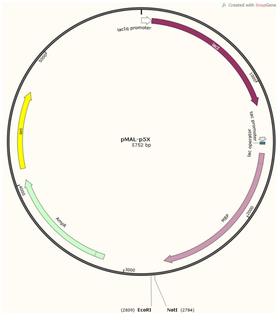
Figure 84: pMAL-p5x vector used in the work in this chapter. pMAL-p5X 5752bp, ampicillin resistance, lacIq promoter Linearised by EcoRI recognition sequence GAATTC and NotI recognition sequence GCGGCCGC. Digest products were a 25bp cut out region and 5727bp linearised vector. The parent vector of pMAL-p5X is pUC18. This figure was created using the SnapGene software (from Insightful Science; available at www.snapgene.com ).
