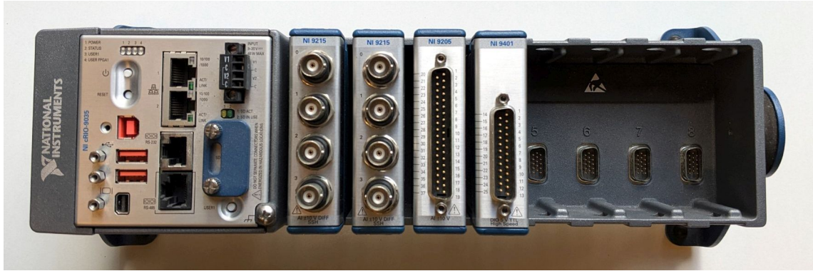
Figure 6.16: National Instruments CompactRIO 9035 embedded controller.
