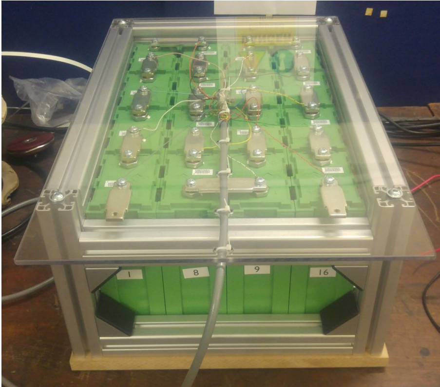
Figure 6.1: Battery pack composed of sixteen series-connected K2B3V90E modules. Approximate dimensions (L×W×H): 650×425×290 mm.
