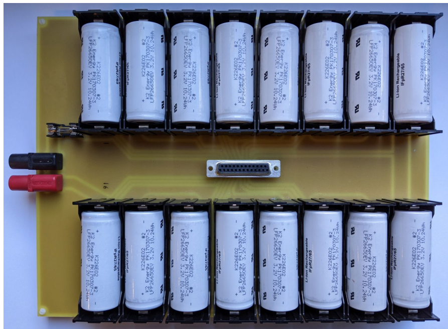
Figure 6.2: Battery pack composed of sixteen series-connected K226650E02 cells on be-spoke PCB. Approximate dimensions (L×W): 286×219 mm.
