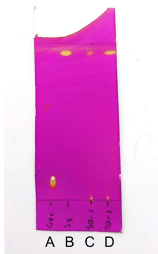
Appendix 3.2: Thin-layer chromatography plate for S-Ger analysis to detect any unreacted geraniol and/or elemental sulfur where A: geraniol, B: elemental sulfur, C: S50-Ger D: S70-Ger using 1:1 hexane:ethyl acetate as the eluent.
