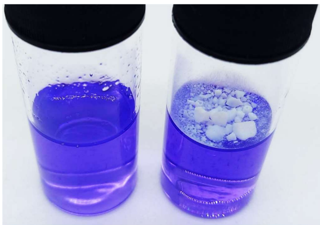
Figure 4.16: Photograph of vials containing unmodified fumed silica (left) and HMDS-modified silica (right) dispersed in water dyed with Brilliant Blue R.
