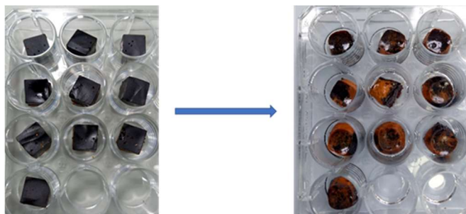
Figure 2.29: A photograph of S70-PA before (left) and after 24 h incubation in water at 35 °C (right) for the leaching study.
