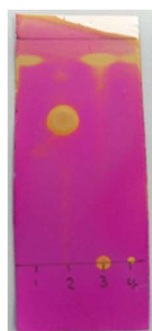
Figure 2.31: Thin-layer chromatography plate for S-PA analysis in order to detect any unreacted perillyl alcohol and/or elemental sulfur where 1: elemental sulfur, 2: perillyl alcohol, 3: S50-PA 4: S70-PA using 1:1 hexane:ethyl acetate as the eluent.
