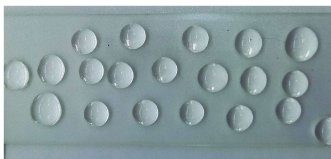
Figure 4.5: Photograph of glass spray coated with S50-PA nanoparticles after heating at 140 °C.
