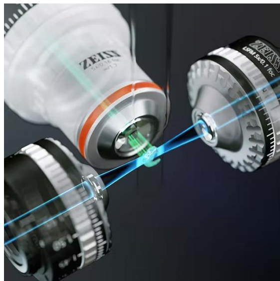
Figure 1.7. Demonstration of light-sheet illumination on a 3D sample using the Zeiss Z.1 light-sheet microscope. The sample is mounted in a column of low percentage agarose that enables the sample to be held in position for imaging (Zeiss, 2022)
