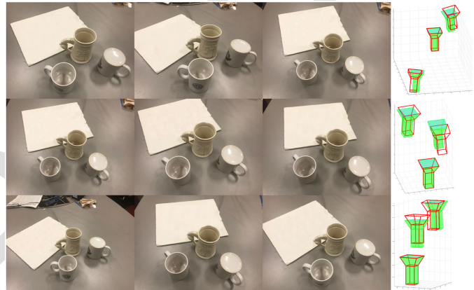
Fig. 11. Trifocal relative pose results for a dataset comprising three mugs, which is challenging for traditional sfm. Each shows images with ground truth (green) and estimated poses (red outline).
