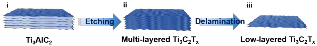
Figure 3.1 Schematic illustration of the low-layered MXene nanosheet synthesis process.
