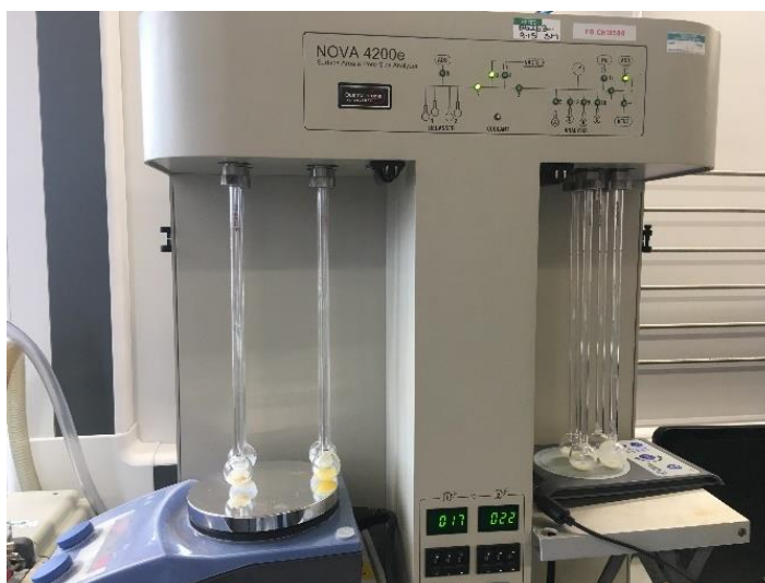
Figure 3.3: Quantachrome Nova 4200e and configuration used to measure gas uptake in liquid samples.
