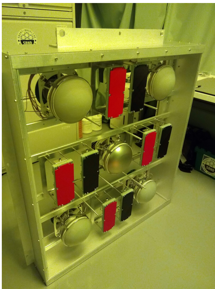
Figure 3.7.: Image of a PDS box showing the position of the 5 PMTs and the 4 pairs of X-ARAPUCA'S. The central PMT is left uncoated, whilst the 4 outer PMTs are coated with TPB.
