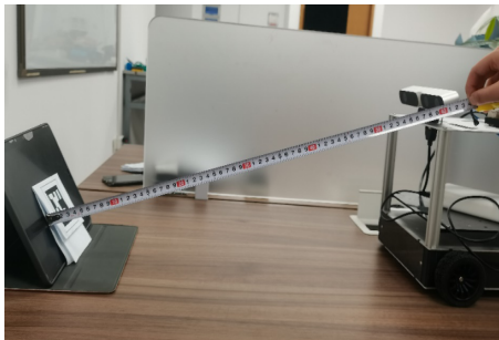
Figure 6.8: Distance between an AGV and Apriltag
