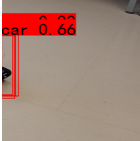
Figure 5.10: Duplicate detection in Faster RCNN
