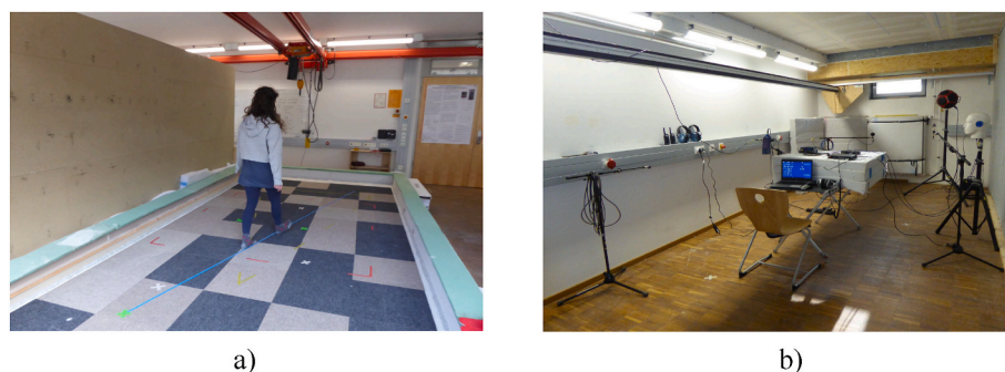
Fig. 1. Impact sound recordings in the laboratory: a) an adult walking on the floor sample in the source room, and b) the receiving room equipped with microphones and sound absorbing panels.
