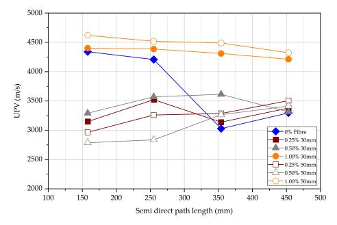
Figure 15. Semi-direct UPV measurement vs. path length at 3 days.
