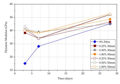
Figure 21. The modulus of elasticity (GPa) of beams at 3, 7, and 28 days.
