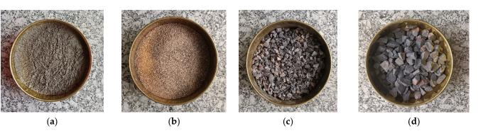
**Figure 2.** (a) Commercial cement; (b) river sand; (c) natural coarse aggregates (NCA)—10 mm; (d) natural coarse aggregates (NCA)—20 mm.
