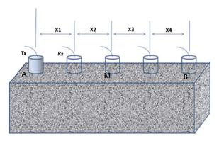
Figure 7. Schematic view of Indirect UPV test.
