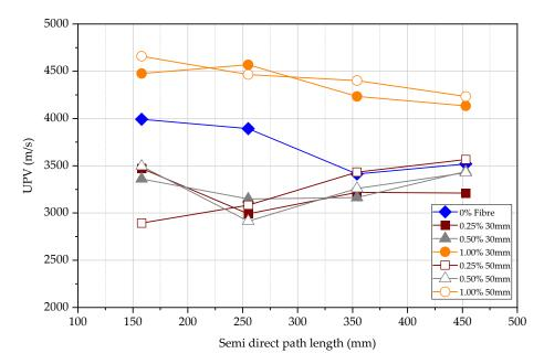
Figure 16. Semi-direct UPV measurement vs. path length at 7 days.
