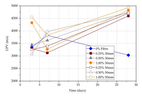
Figure 14. Semi-direct UPV measurements at 3, 7, and 28 days.
