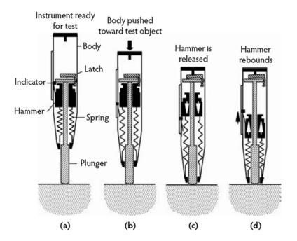
Figure 3. Operation of the rebound hammer.
