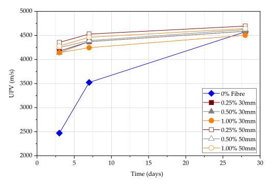
Figure 11. Direct UPV measurements at 3, 7, and 28 days.
