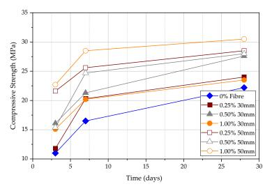
Figure 9. Compressive strength (MPa) using rebound hammer test result.
