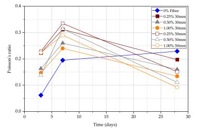
Figure 22. Poisson's ratio of beams at 3, 7, and 28 days.
