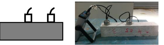
Figure 6. Indirect UPV measurement.
