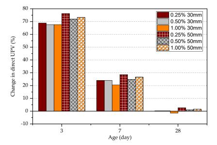
Figure 12. Change in direct UPV in FRC relative to plain concrete.
