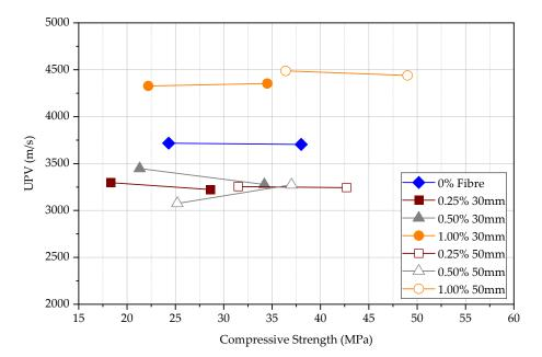
Figure 17. Semi-direct UPV measurements vs. compression strength.
