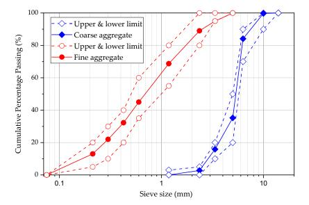
Figure 1. Sieve analysis data of coarse and fine aggregates.
