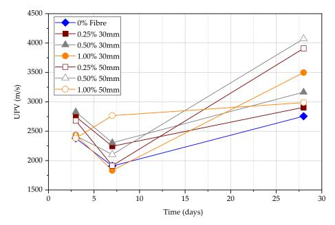
Figure 19. UPV indirect measurements with 200 mm path length.
