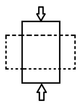
Figure 20. Length change of material under compression.
