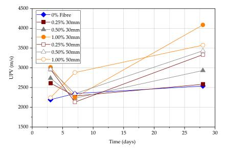
Figure 18. UPV indirect measurements with 100 mm path length.
