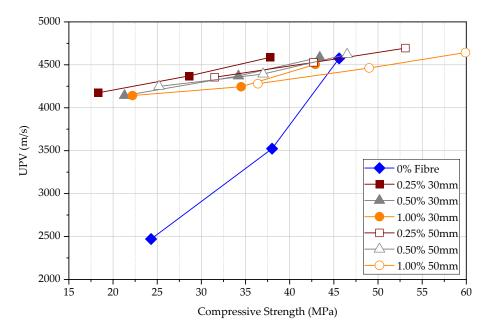
Figure 13. Direct UPV measurements vs. compression strength.
