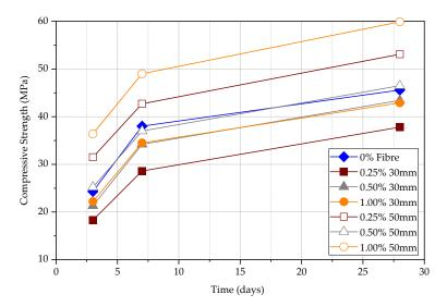
Figure 8. Compressive strength for different fibre content at 3, 7, and 28 days.
