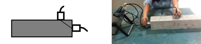
Figure 5. Semi-direct UPV measurement.
