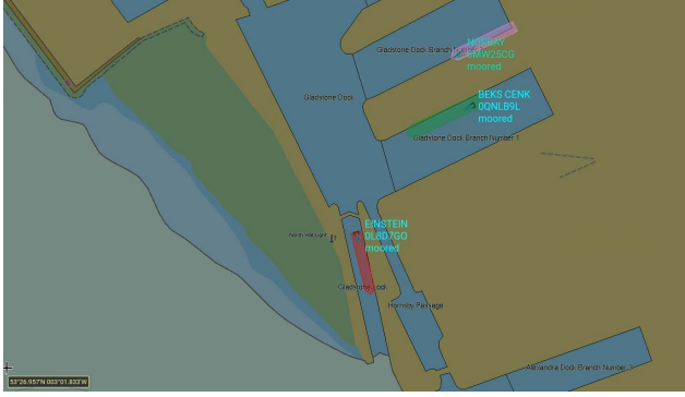
Fig. 2. Three moored vessels. The vessels and the detections are depicted on the map of the iVision VTS system of Denbridge Marine Ltd. The first line of the label contains the ship's name, the second line shows the track id, and finally the third line shows the phenomenon detected.
