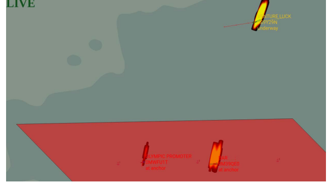
Fig. 3. Two vessels at anchor (lower part), and a vessel underway (top part). The red polygon corresponds to an anchorage area, while the shapes around the vessels correspond to radar blobs.
