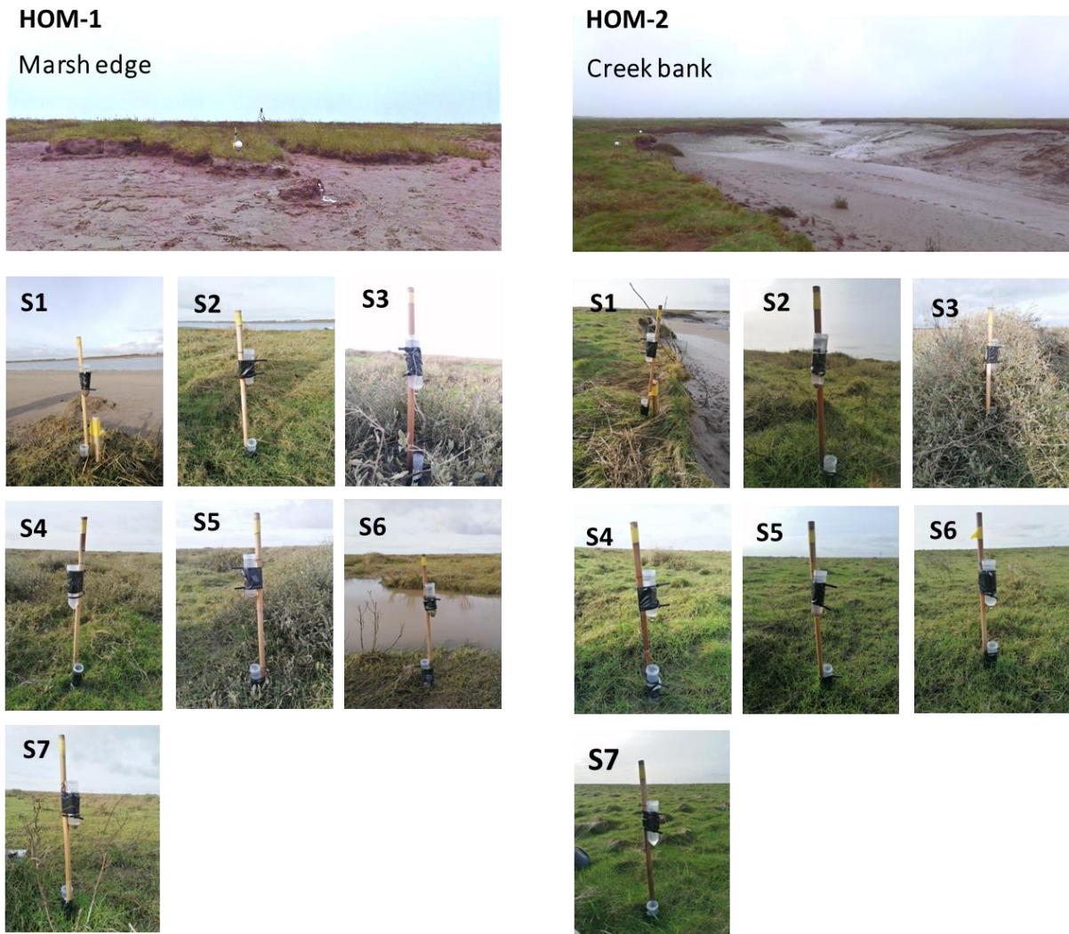
Figure S10. Panoramic of the starting points of the transects HOM-1 (marsh edge) and HOM-2 (creek bank) obtained with a FARO 3D laser scanner Focus X330 and photos displaying the locations of the sediment traps along each transect.
