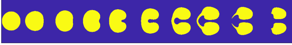
Figure 3.6: Droplet ‘bag’ breakup for We = 38.7 . The flow direction is from left to right.
