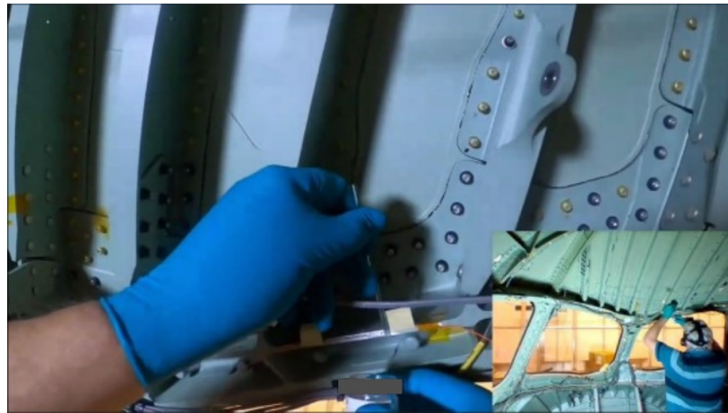
Figure 4. Installation of a sensor unit in the full-scale fuselage test, from [8].
