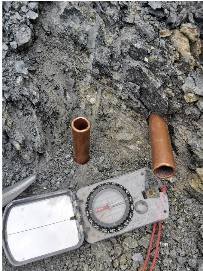
Figure 2.10: Two copper tubes that were used to collect oriented samples of fault gouge from an area cleared of weathered top soil. Compass clinometer for scale.
