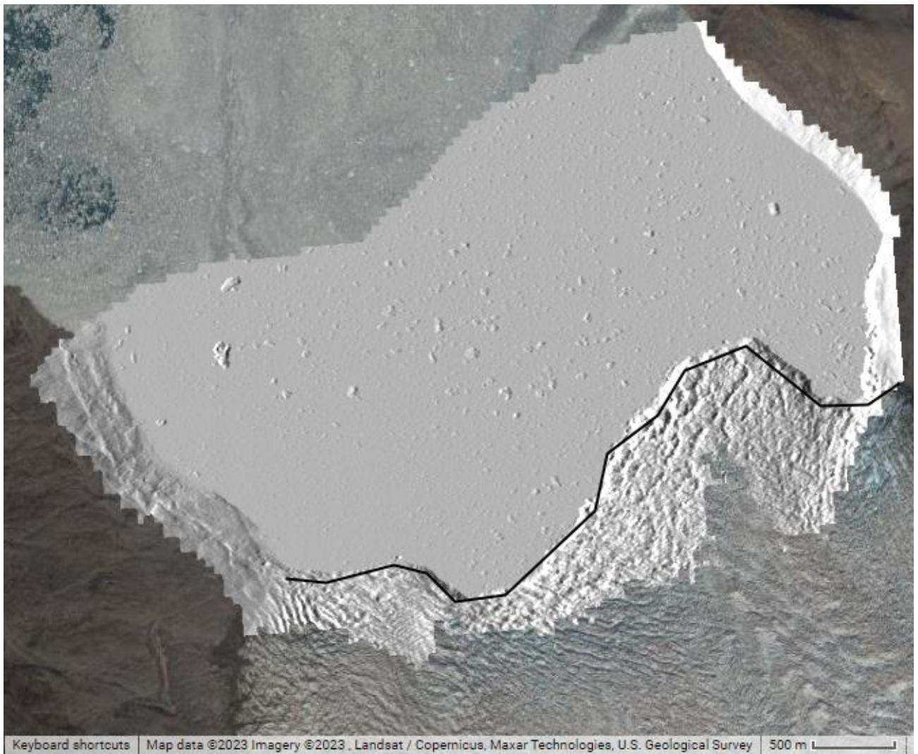
Figure S3. Example of the automated ROI construction with the filtering of the closest terminus trace by date (shown by the black line) overlaying the clipped ArcticDEM tile for automated iceberg detection at KNS.
