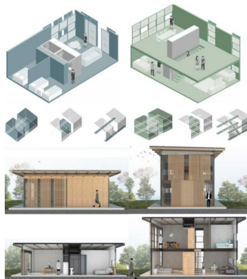
Figure 3. Adaptable layout of a parametric modular system.
