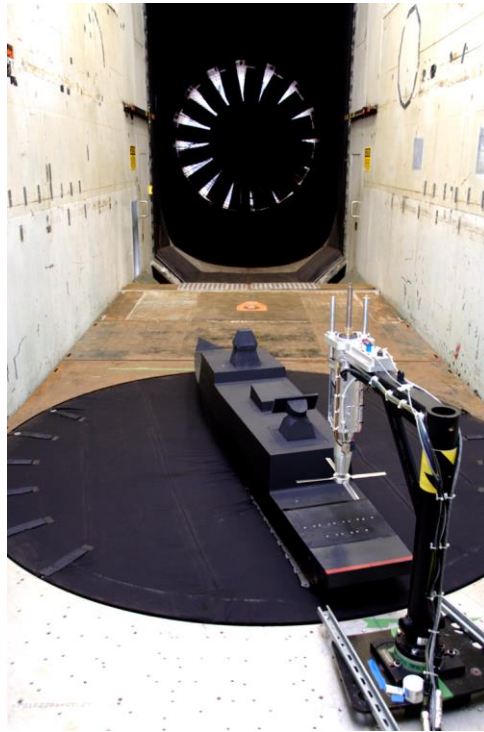
Figure 8: Test setup for ship motion experiments in the NRC 3 m x 6 m Wind Tunnel. The rotor-only HULMS is shown behind the NATO-GD model, 1:50 scale.
