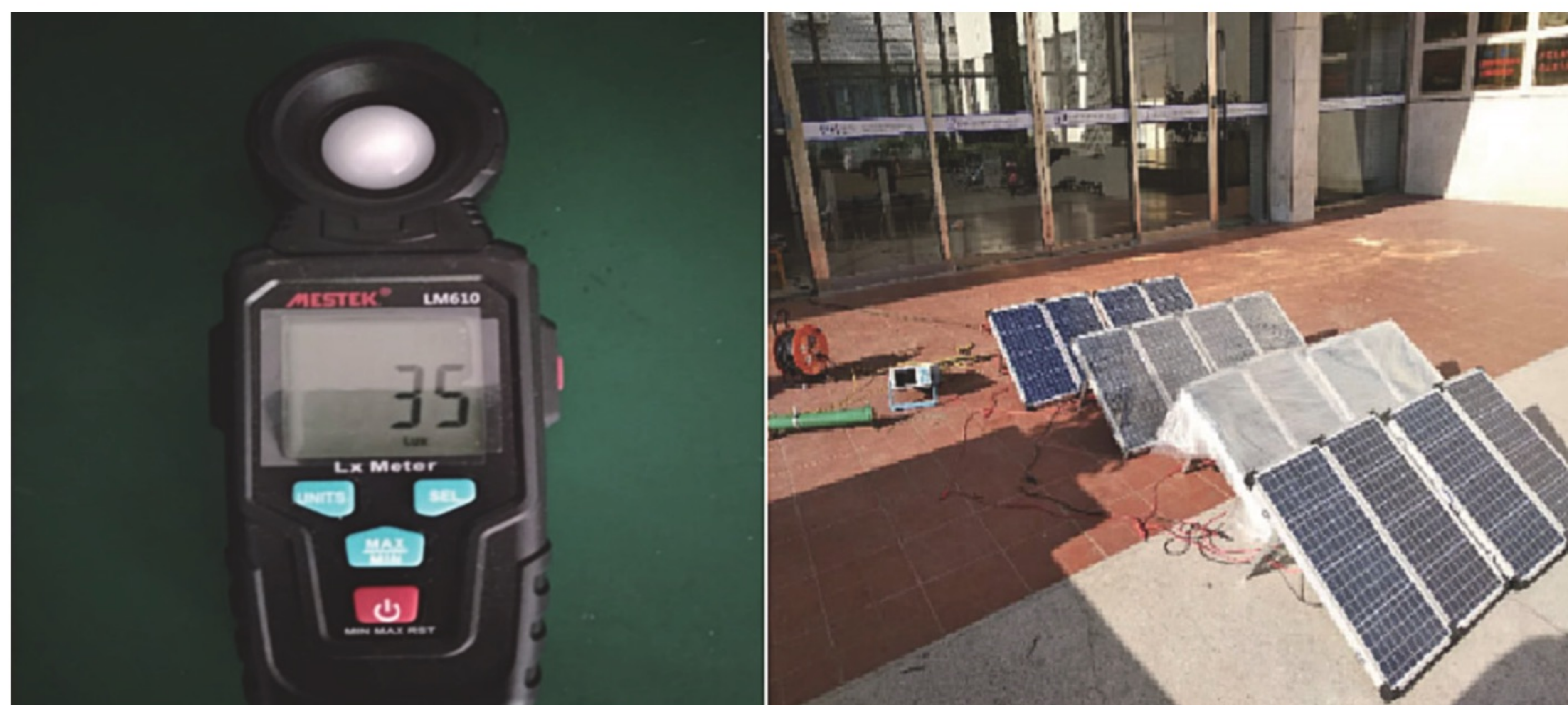
Fig. 7. Actual shading implementation of the 4 \times 4 array.
