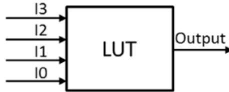
Figure 1.18: Simple 4-input Look-up Table (LUT) logic block. From [80]
