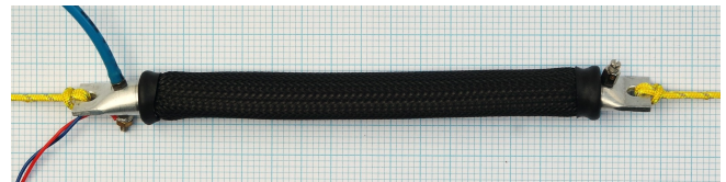
Fig. 1. Prototype of the SMA valve McKibben-based PAM with passive exhaust orifice.
