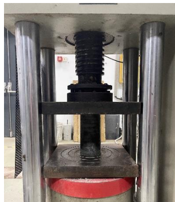
Figure 4. Compression test on cylinder specimens
