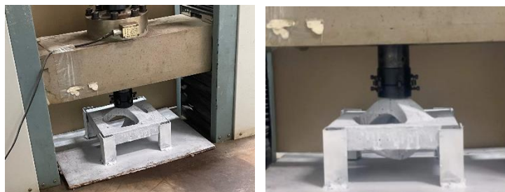
Figure 7. Load testing on the façade specimen
