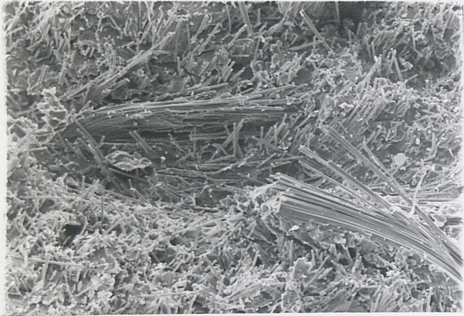
Figure 3.45 fracture surface containing fibre bundles mag.=80 x
