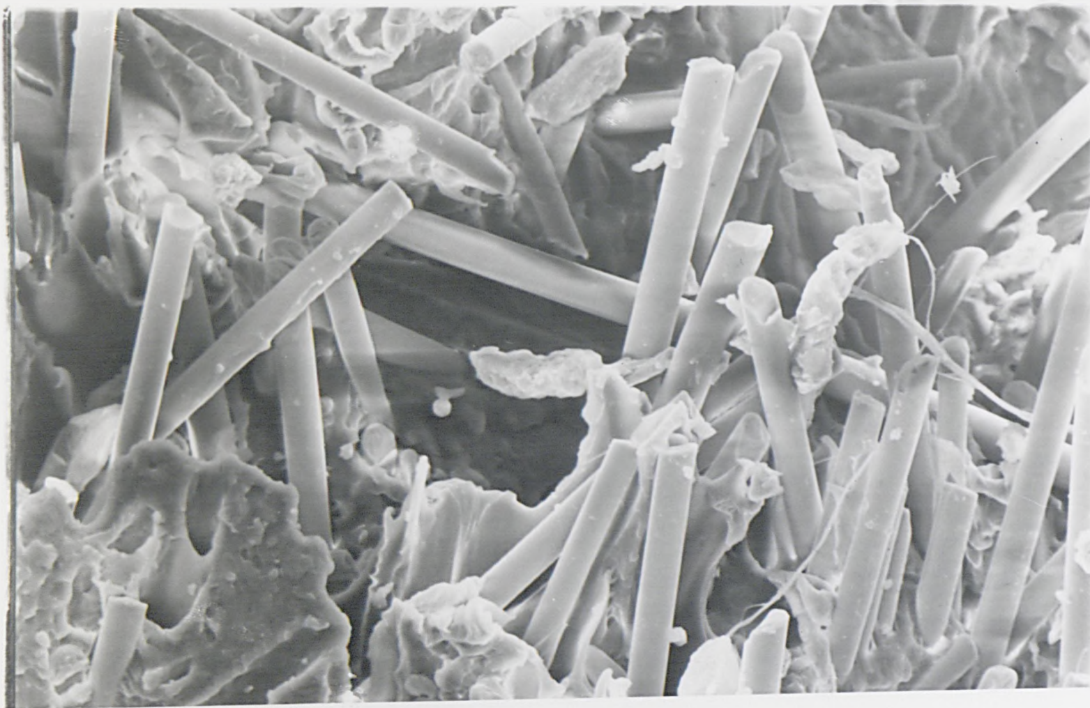
Figure 3.58. stereoscan photograph of 'boiled' fracture surface mag.=768x - MSS 1640 sized fibres
