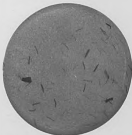
FIG. 3.55 INFLUENCE OF MOULDING VARIABLES ON FIBRE DISPERSION
