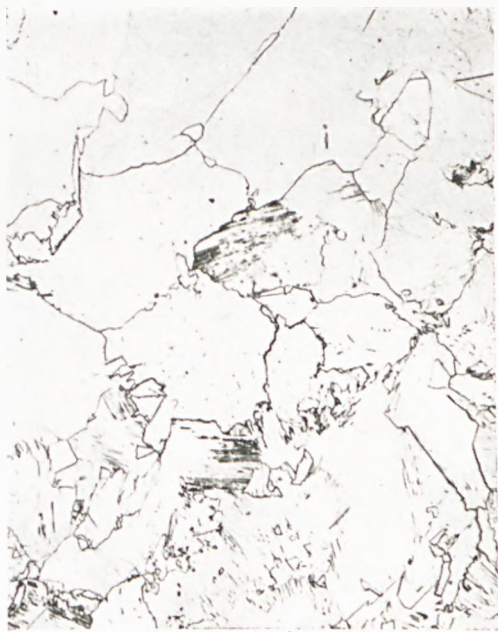
Fig. 18. A Cu-Ga (25.4% Ga) eutectoid alloy in which the entire structure is massive \zeta . Obtained by quenching from 775°C. 19 100X.
