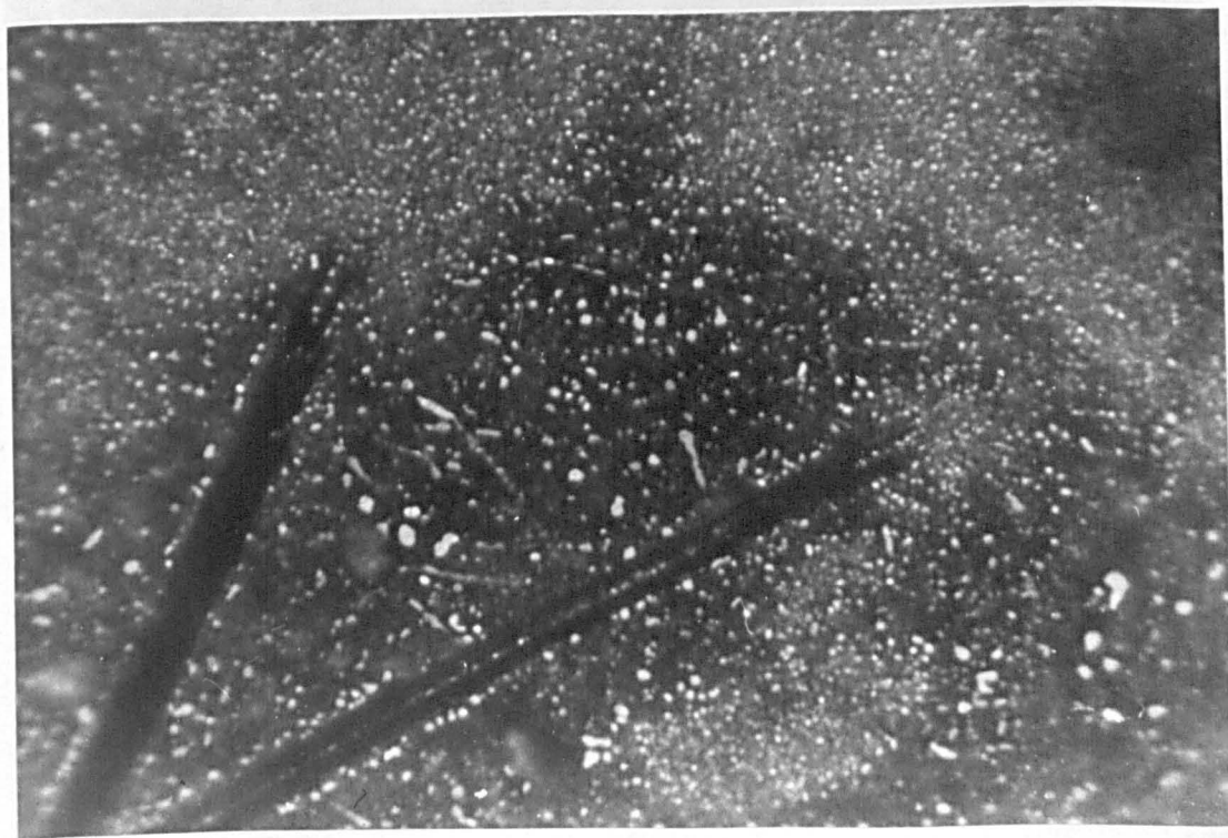
P. 4.9 The alteration in glass after 24 hrs at 1000°C in air, showing variation in alteration size and unaltered feldspars
